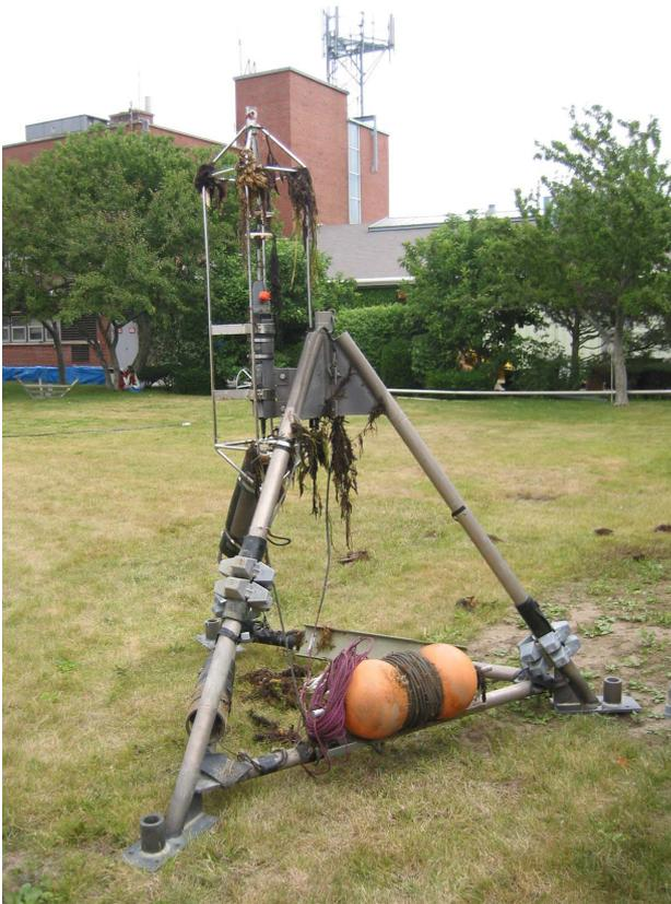
Fig. 1. Wave tripod with MAVS current meter, one of two Pop-Up recovery floats, and two acoustic command releases, after recovery from Vineyard Sound. Seaweed on the protective mooring cage seldom affected the measurement of waves and current during the 51 day deployment.
