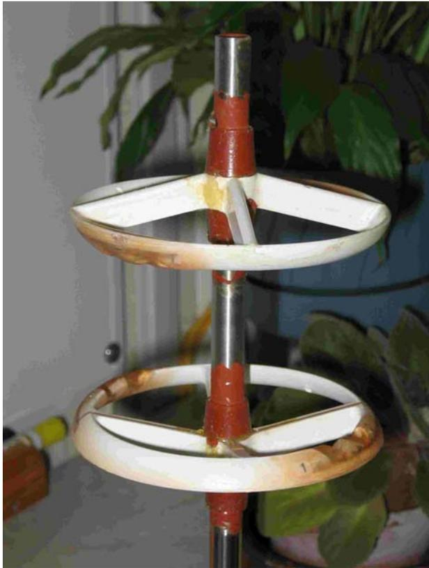
Fig. 3. MAVS velocity sensor for an elevation of about 15°. The acoustic paths are only shadowed by one of the upper struts, a short section of the upper ring, and the central support tube.
