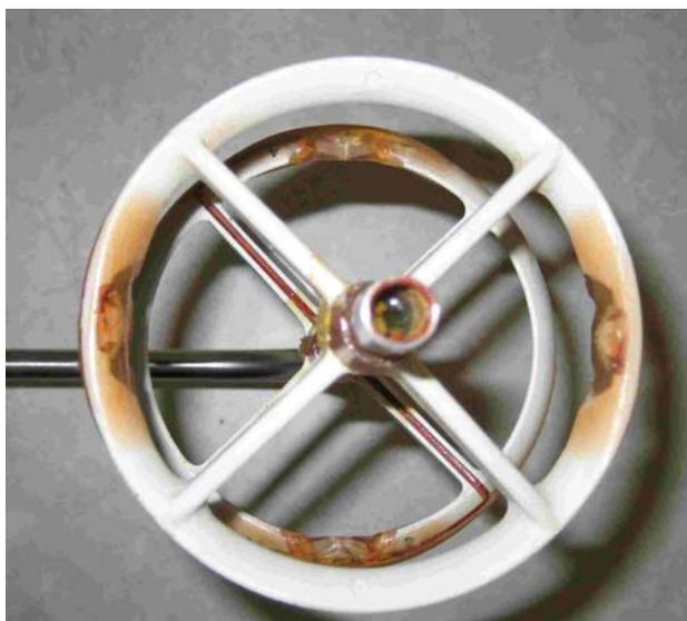
Fig. 2. Velocity sensor viewed on axis. This is a bent sensor showing the struts supporting the rings but the housing is off to the left. This view is that seen by the flow at 90° elevation.
