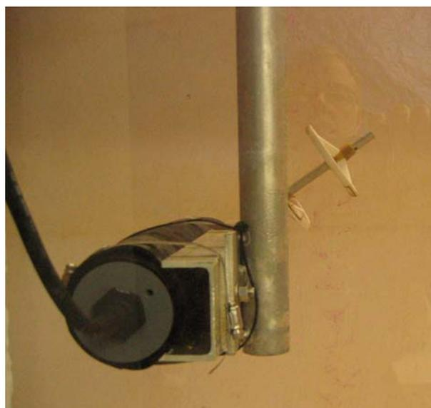
Fig. 5. Bent sensor MAVS being towed with a 45° elevation angle of the sensor to the tow direction. Permanganate crystals have been dropped to streak the water in the flume so the displacement of fluid after passage of the sensor can be seen, barely visible here.
