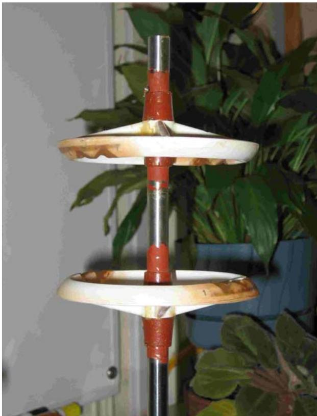
Fig. 1. MAVS velocity sensor. The faired rings are 118 mm in diameter, separated by 70 mm, each supported by four struts from a central support tube 12.5 mm in diameter. This view is that seen by flow at 0° elevation
