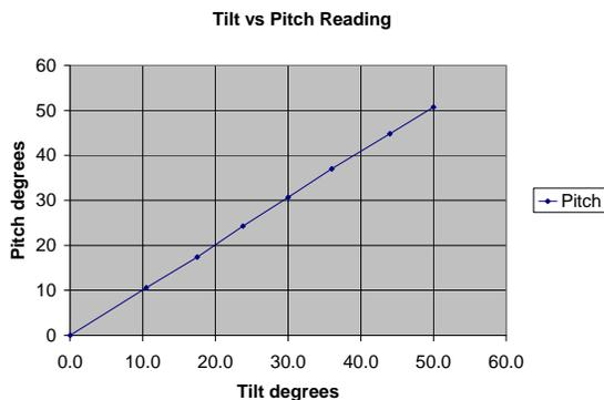
Fig. 1. Applied tilt angle and measured pitch derived from 5 digitizations of the ADXL202 duty cycle output. The scale factor was chosen for a best fit.
