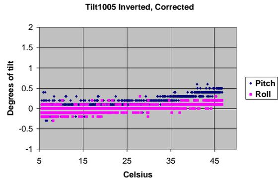
Fig. 9. Temperature compensation is effective with the sensor inverted as can be seen with the temperature run of tilt sensor 1005.
