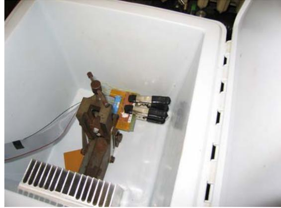
Fig. 4. The thermoelectric cooler with temperature calibrating board contains six ADXL202 tilt sensors under a copper bar held in close contact with clamps. A thermistor is inserted into a hole in the bar and coupled to it with heat sink grease. The machinist vise is set to hold the tilt sensors horizontal during the calibration. For descending temperature, the cooling fins sequester moisture so the circuits remain dry.
