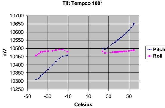
Fig. 3. Temperature coefficient measurements made with heat gun and circuit cooler. The region of oceanic interest is inaccessible due to condensation of moisture on the circuit.
