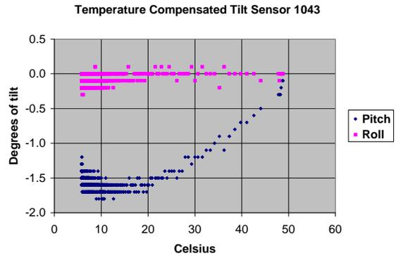
Fig. 5. Tilt was zeroed at 48°C and the temperature was reduced to 5°C in the thermoelectric cooler. Between 24°C and 5°C the pitch and roll readings were within 0.3° tilt angle of the coefficient-determining settings at 16°C and 5.5°C.
