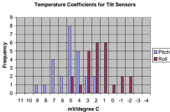
Fig. 7. Temperature coefficients for twenty ADXL202 devices show a spread of values. No single coefficient can be used and pitch and roll for each device must be obtained.
