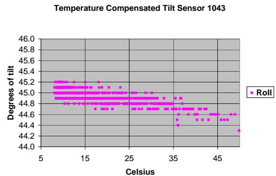
Fig. 6. There is negligible effect of temperature coefficient on the scale factor. This tilted temperature run shows less than 0.3° of tilt uncompensated between 30°C and 8°C.
