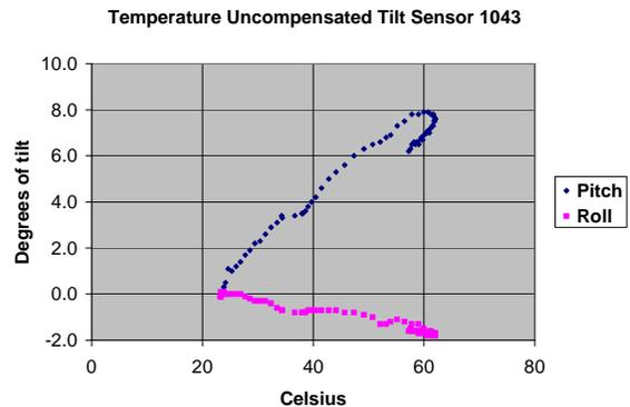
Fig. 2. Tilt appears to increase as much 8° with an increase in temperature from 25°C to 60°C from an uncompensated tilt sensor. Heat was applied with a heat gun while the sensor was clamped in a horizontal orientation. Hysteresis in the tilt measurement, when the heating stopped, results from the separation of the thermistor from the tilt sensor causing a temperature tracking error during rapid heating.
