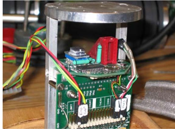
Fig. 8. Attitude module with the three-axis magnetometer compass and the two-axis tilt sensor. There is a right angle DIP socket to mount the ADXL202 circuit into if the MAVS current meter is to be deployed horizontally.
