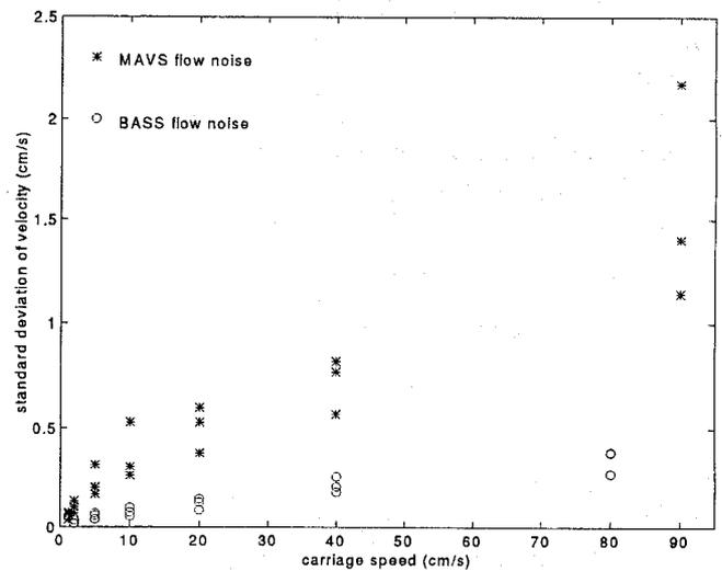
Fig. 7. Measured flow noise of BASS and MAVS sensors towed through still water.
