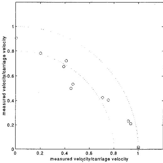
Fig. 5. BASS cosine response to rotations about the perpendicular axis.
