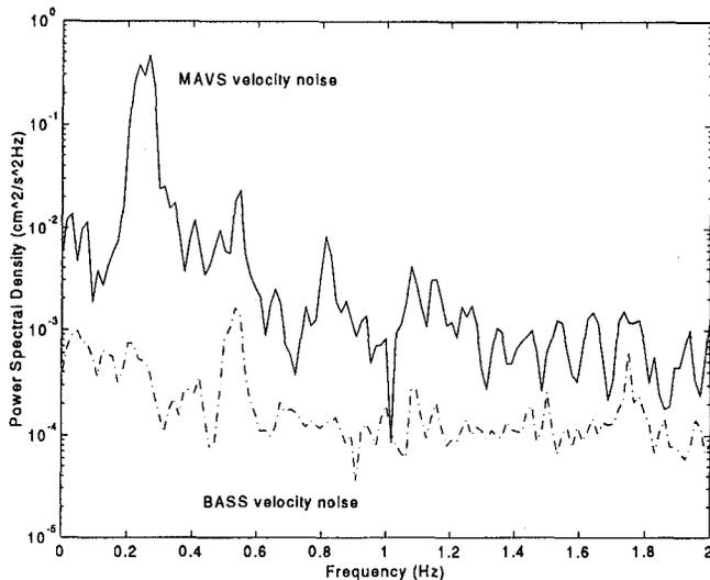
Fig. 8. Noise spectra of velocity in direction perpendicular to both tow velocity and axis of radial symmetry. Tows at two centimeter per second through still water.
