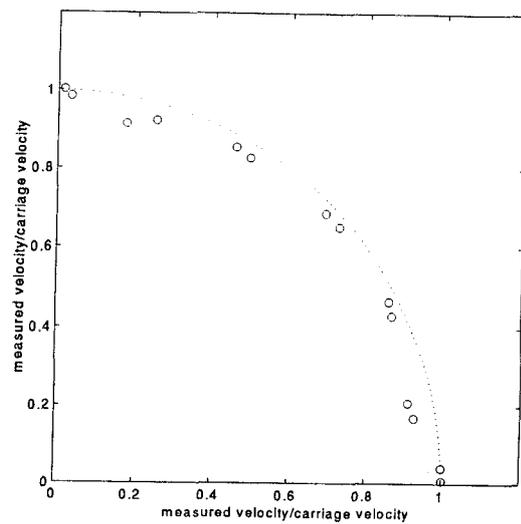
Fig. 3. BASS sensor cosine response to rotations about the longitudinal axis.
