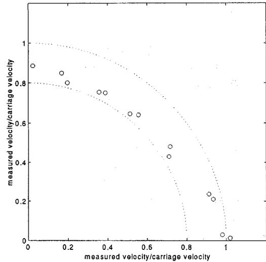
Fig. 6. MAVS cosine response to rotations about the perpendicular axis.
