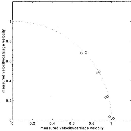
Fig. 4. MAVS sensor cosine response to rotations about the longitudinal axis.
