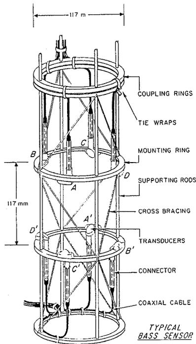
Fig. 1. Typical BASS sensor showing acoustic transducers, braced frame, and external electrical cables.
